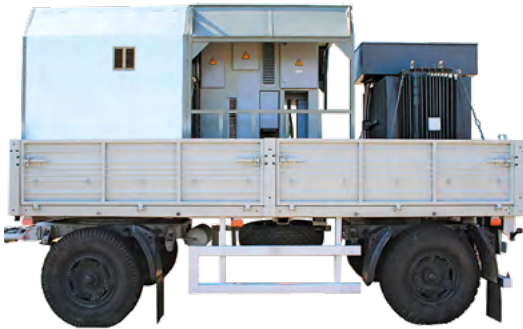
MCU-2-05/1000-630 based on drop-side trailer MAZ 8926-017-02
